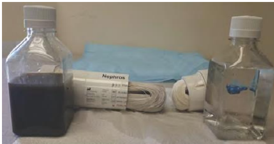
Typical removal results of a Nephros filter.
